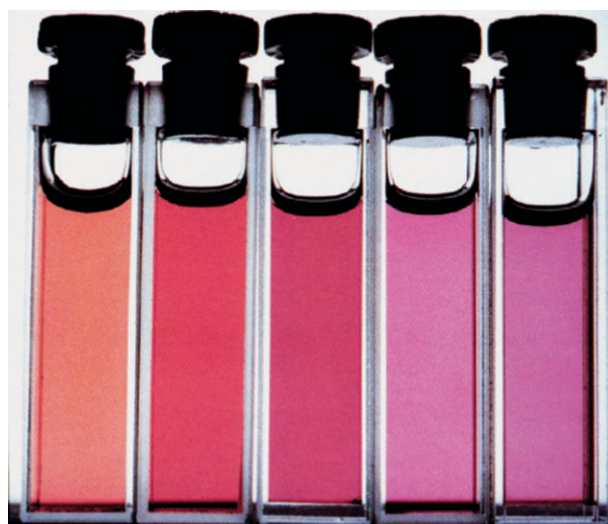
Fig. 2 Changing in the plasmon peak position induced by varying the solvent refractive index. Refractive indices of the solutions at the absorption band maximum are 1.336, 1.407, 1.481, 1.525 and 1.583, respectively. 32 Reprinted with permission from Langmuir , 1994, 10, 3427. © 1994, American Chemical Society.
